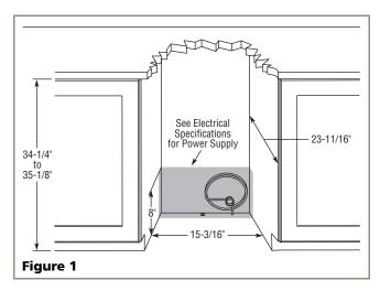
Follow the cut-out drawing in **Figure 1**. The 15-3/16" width allows 1/4" for ease in installation and removal of the unit. 24" is the counter depth in most installations. The unit is 23-11/16" deep including the handle on Black and White models and 23-11/16" deep including the door and *not* the handle on Stainless Steel models (see **Figure 2**).
